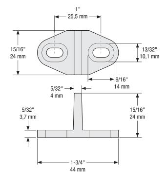
Fasteners: (2) Phillips Screw, 5/32" x 1-3/8" Long, Self Tapping (2) Anchor, 5/16", Plastic
