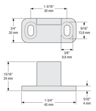
Fasteners: (4) Phillips Screw, 5/32" x 1" Long, Self Tapping (4) Anchor, 5/16", Plastic
